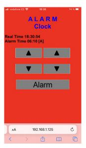
Use the left up/down buttons to set the hour of alarm time, and the right up/down buttons to set the minutes.
